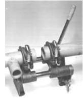
Move the pipe ends together until they are almost touching, then check for misalignment (maximum allowable misalignment is 10% of wall thickness). Tolerances on small bore pipes should be sufficient to permit pipe alignment in the MV70 without adjusting the clamps. However, in severe out of round situations, adjust out any misalignment by loosening the clamps and rotating the pipes, and/or using packers as necessary.
