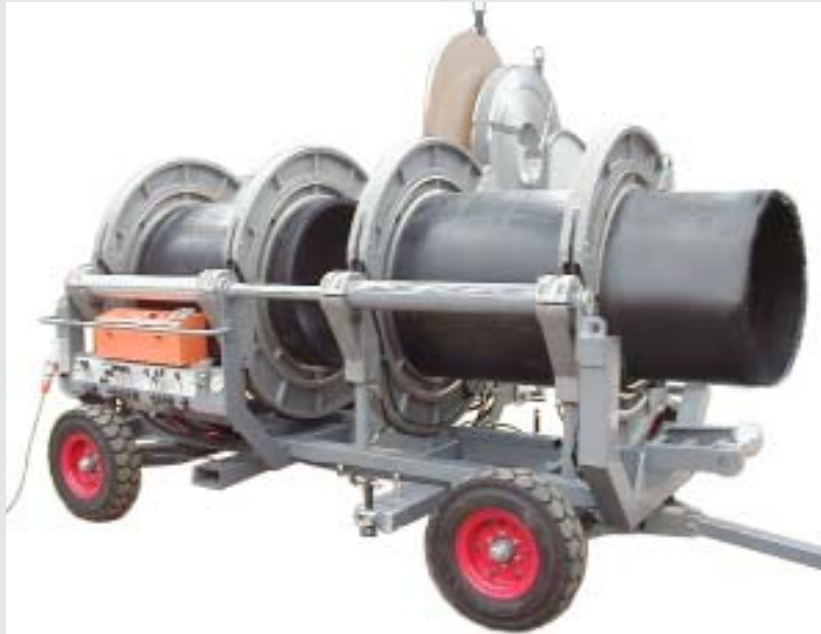
butt welder for pipe and fittings - 1000mm to 630mm
